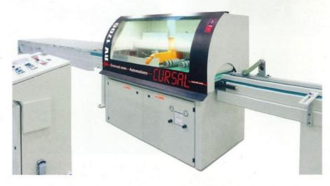
traction system with specific pressure wheels – rubbered and anti-slip at a reduced distance – guarantees speed, precision, and an uniform pressure on the entire surface of the board.
