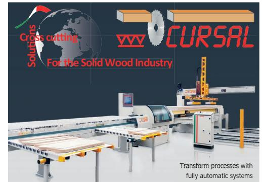
Full optimization with integrated cross-cutting from sawmill to window sector Optical scanner for quality and defects detection
